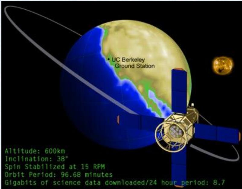
The orbit is inclined ( $38^\circ$ ) – passages through radiation belts and South Atlantic Anomaly (SAA)
