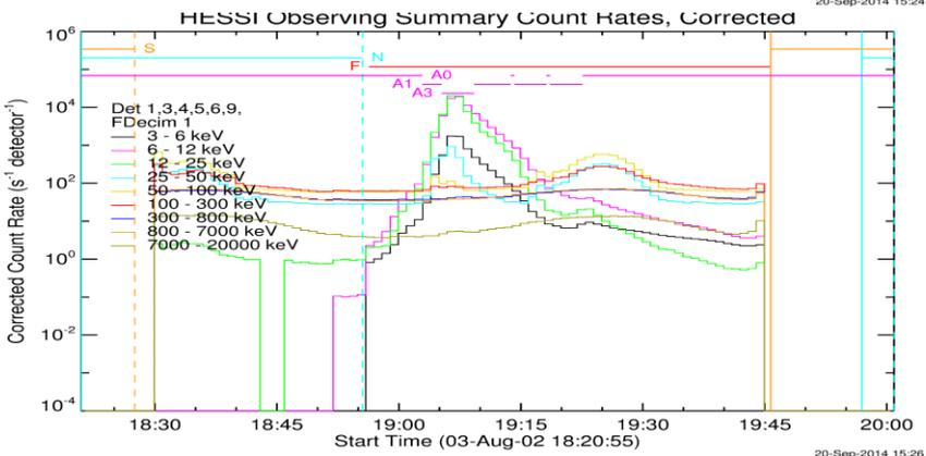
The flare list is obtained by comparing the observing „corrected” count rate in the 6 to 12 keV energy band to a threshold obtained using a 60 second running average.
