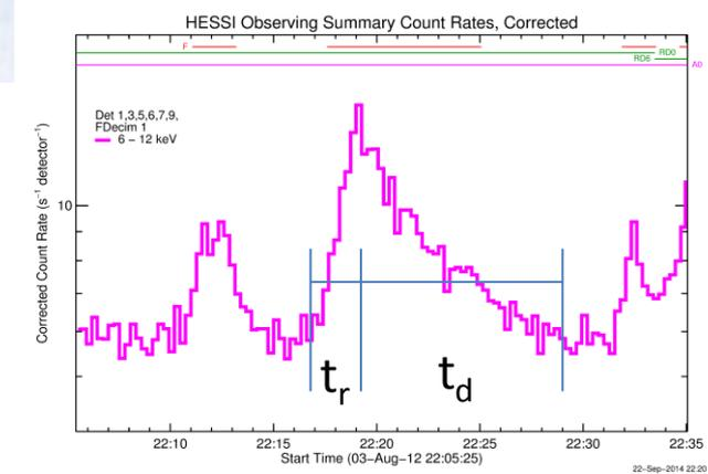
$$A = \frac{t_{delay} - t_{rise}}{t_{delay} + t_{rise}}$$
