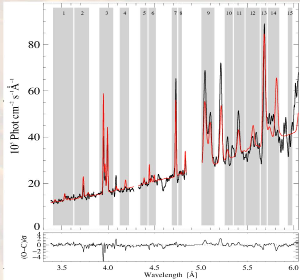
RESIK spectra were fitted with a use of Withbroe-Sylwester algorithm for a number of accumulated spectra
