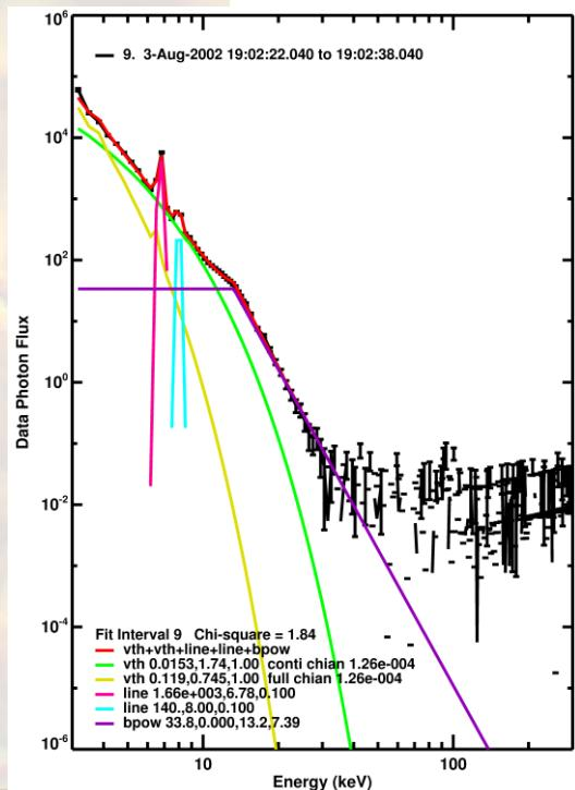
RHESSI spectra were fitted with two thermal components, two gaussians and broken power-law.
